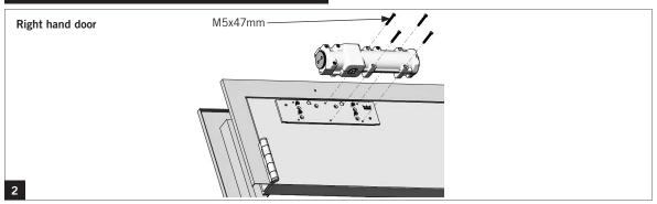
NOTE: Orient pinion closest to hinge.
