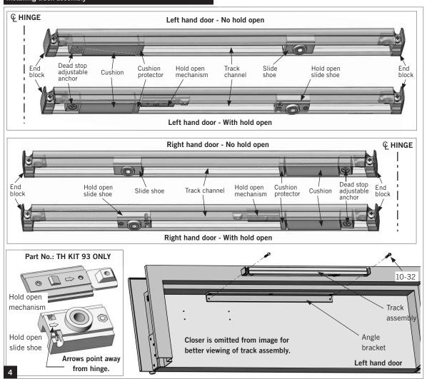
4.1 Position individual components inside track channel and screw down each fitting with a Phillips flat head driver.
